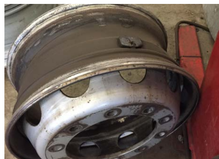
Afb. 0.4: TPMS sensor in diepbed.
